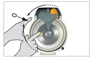
To adjust, press in the button and revolve the winding disc in the appropriate direction.
