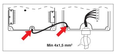
The power supply to the feeder must not be disrupted when the weaving machine stops.
