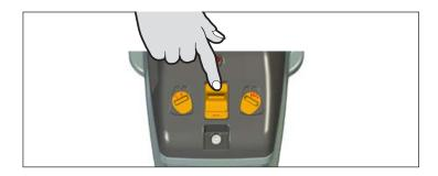
Grip the winding disc and, whilst pressing the orange button on the front of the spool body, rotate the disc until the button is felt to locate. Aligning the mark on the winding disc with the line on the motor house gives the zero separation position.
