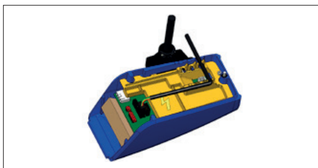
Position the cable as shown then re-assemble the circuit board housing onto the feeder.
