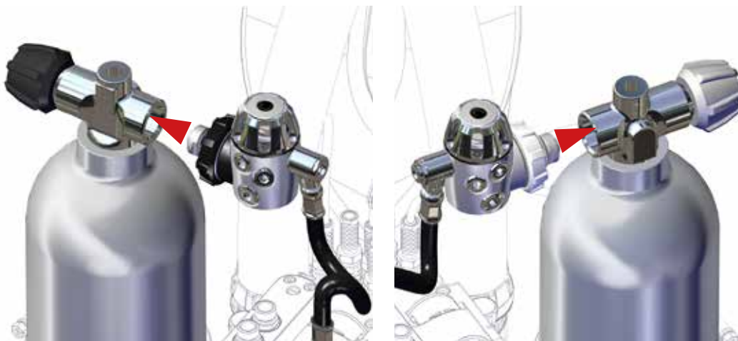
Figure 1-39. Align the diluent regulator with the diluent cylinder female DIN thread. Push it in and hand tighten the diluent regulator swivel nut.
