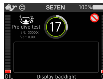
Figure 2-5. Test 17 (Backlight Power consumption), displaying test number in the center circle, progress is shown through the inner green circle moving counter clockwise.
