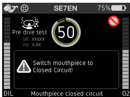
Figure 2-10. Test 50 – Closed-Circuit mouthpiece position.
