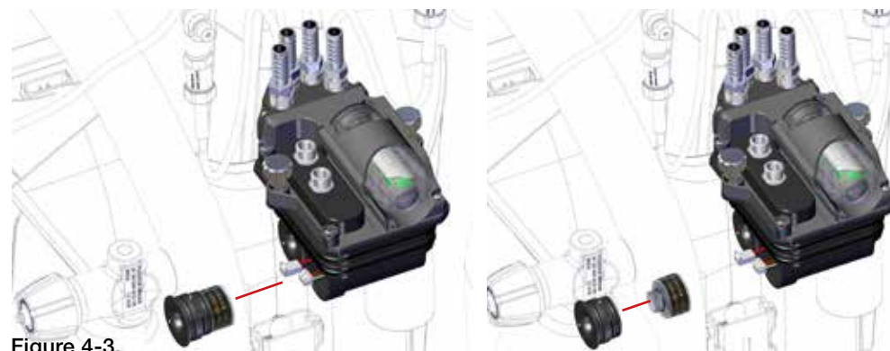
Figure 4-3. Solid States O2 sensor removal.
