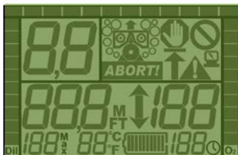
Figure 2-4. The Primary Display showing all LCD elements.
