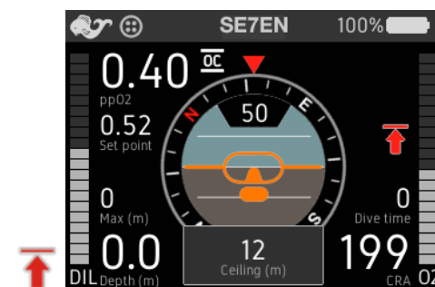
Figure 3-11. Decompression ceiling alert.
