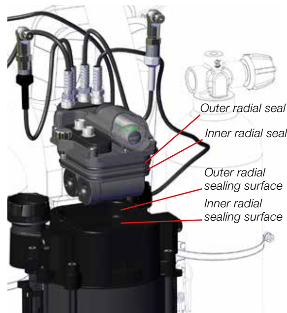
Figure 1-36. Align the cable junction box with the front of the gas processor (closest to backpack), then insert the electronics module into the processor housing
