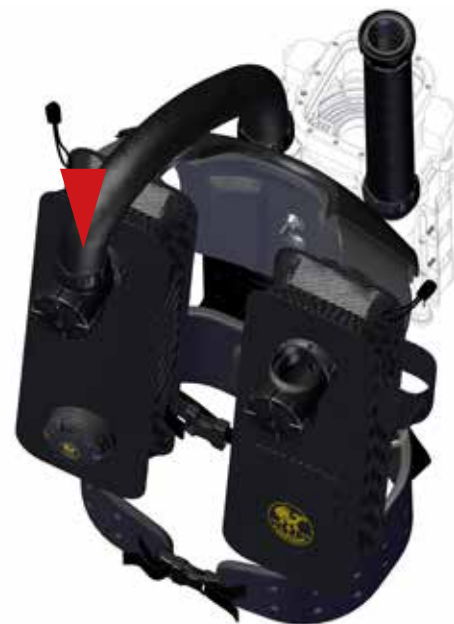
Figure 1-31. Attach the right counterlung water diversion manifold to the right rear breathing hose.
