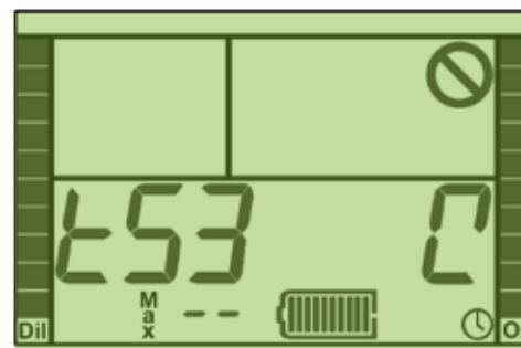
Figure 2-11. Test 53 – Oxygen Sensor calibration.
