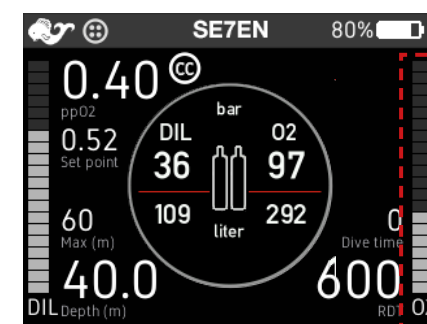
Figure 3-32a. Oxygen cylinder pressure indicator.
