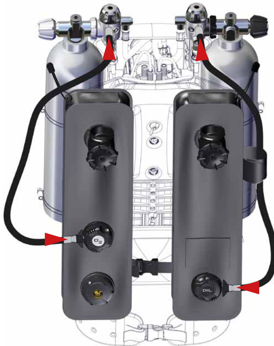
Figure 3-42. LP hose routing.
