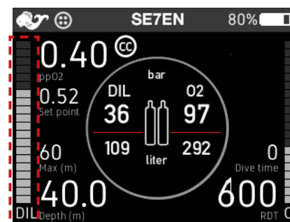
Figure 3-31. Diluent cylinder pressure indicator.
