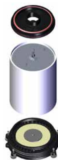
Figure 1-60. Remove the end plate.
