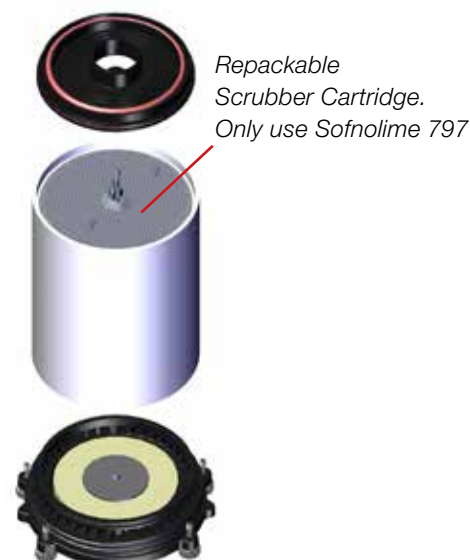
Figure 1-55. The CO 2 Scrubber Cartridge with the Sofnolime® 797.
