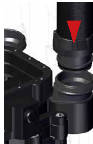
Figure 1-28. Closeup of hose connection.
