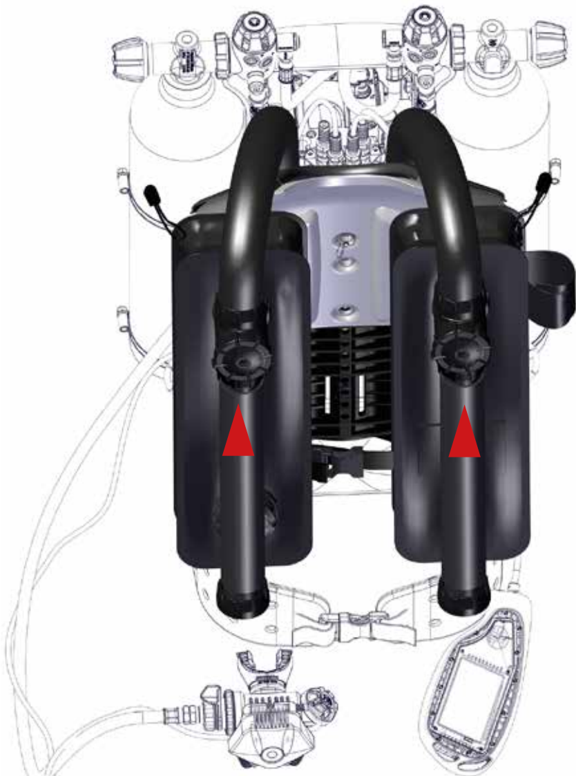
Figure 1-47. Breathing hoses properly connected onto the water diversion manifolds.
