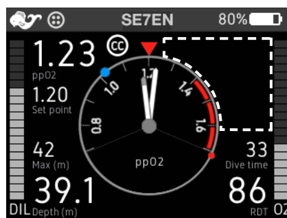
Figure 3-6. Alarm signal area.
