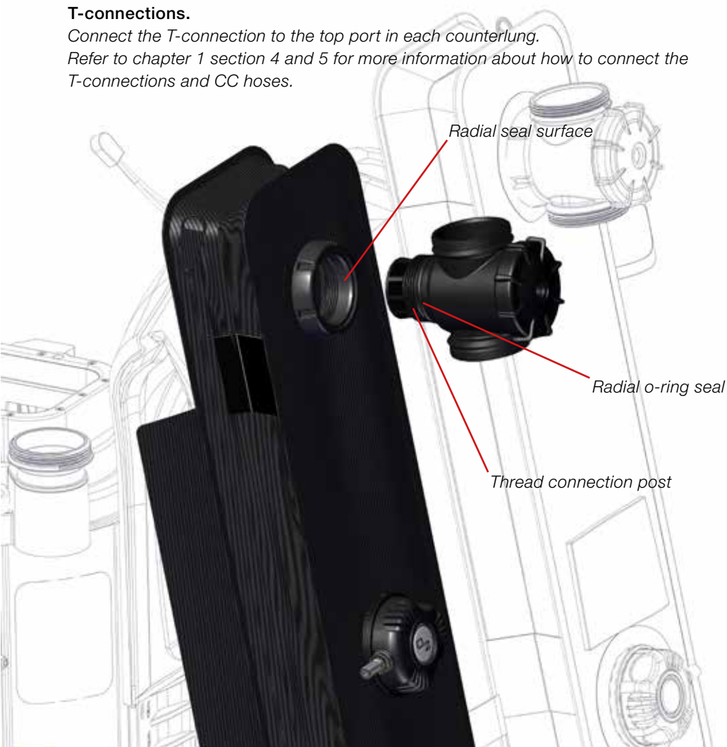
Figure 3-40. Insert the right hand water diversion manifold into the port on the right counterlung. Clockwise tighten the water diversion manifold into the right and left counterlung shoulder port. Note the correct orientation, further described in chapter 1, section 4.
