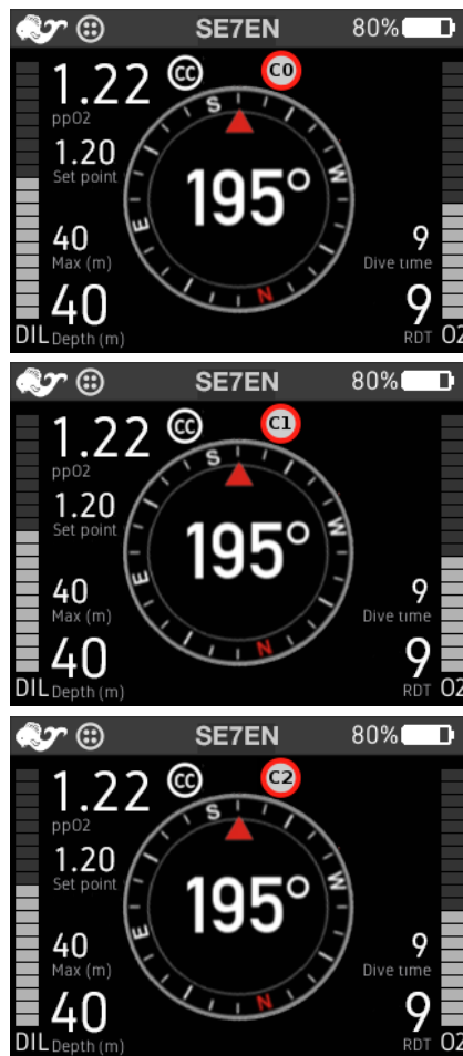
Figure 3-16. Oxygen sensor confidence alerts: C0, C1, C2.
