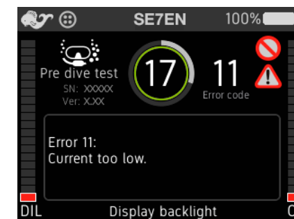
Figure 2-6. Test 17 failure, with flashing error code.
