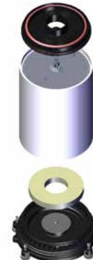
Figure 1-61. Lift and remove the lower sponge; inspect for collected water. Rinse, dry, and store the lower sponge; disinfect if desired.
