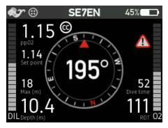
The General alert symbol located in the Alarm Signal Area will flash in synchrony with any other parameter(s) on the screen that is/are inappropriate or out of acceptable range. This signal is intended to catch the diver's attention, and prompt the diver to scan the other elements on the screen to see which value(s) is/are also flashing. As long as one of the other displayed values on the Primary Display is flashing, the General Alert symbol will also flash.
