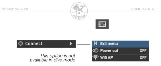
The connect menu is used to connect to external sources such as external sensors, HUD, CPODs and others.
