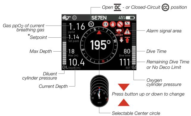
\*In SE7EN dive mode the ppO2 of the breathing loop is displayed while in closed circuit (CC) mode and the ppO2 of the selected OC gas at the current depth is selected while in open circuit (OC) mode.
