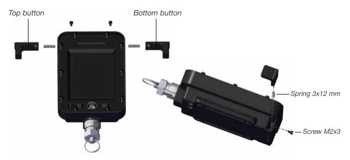
Ensure that the compression spring is correctly re-installed. Hand tighten the screws carefully. The buttons are automatically recalibrated by the M28. Buttons, springs, and screws are available to be ordered as spare parts.
