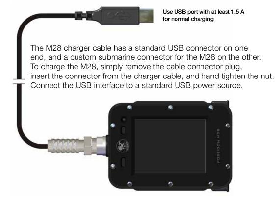
The power source can be any USB connection providing 5.1V and a minimum current of 1.5 Amp. If the LED is flashing alternating green and red for at least 1 minute, it is most likely that the USB power supply's current is insufficient.
