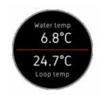
**Temperature.** Displays the current water temperature when you dive. If SE7EN is connected also displays the temperature in your breathing loop. The unit (°C or °F) can be configured in Settings / Temperature unit.
