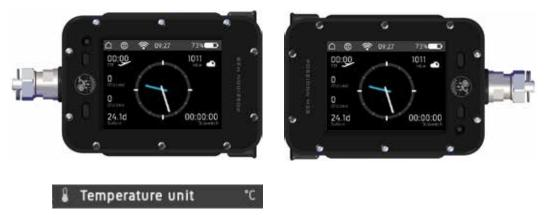
Switch displayed temperature unit between Celsius (metric) and Fahrenheit (imperial).
