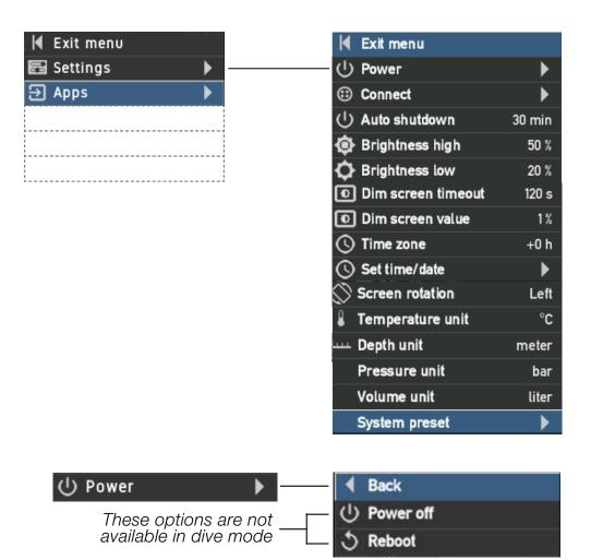
The power menu allows you to turn off the M28 or reboot the M28. If the unit does not power off after a 1 minute, it is also possible to enforce a power off by pressing both buttons for more than 8 seconds.
