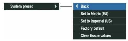
This is a quick way to set all the unit to be displayed into either Metric (EU) or Imperial (US) units. This will only affect the displayed unit settings. Use the "Factory default" to reset the settings back to factory settings. This will not erase any dive log, redbox log or any pictures, only set the settings back to default.
