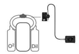
Setup for loop ppO<sub>2</sub> monitoring on any rebreather (CPOD + M28)
