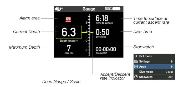
WARNING: The decompression algorithm is disabled in GAUGE MODE.
