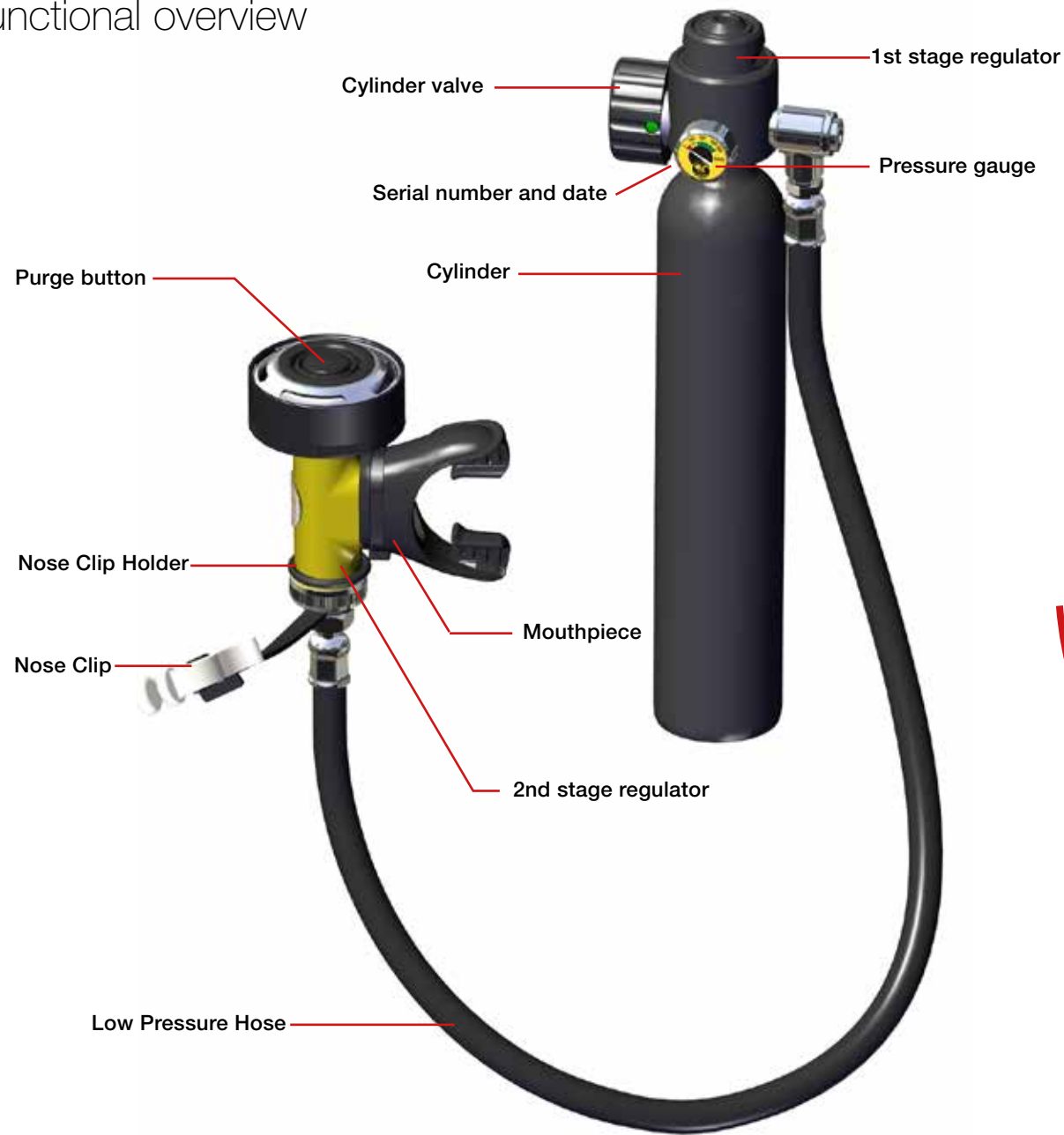
Cylinder valve in position OPEN Turning the valve handle counter clockwise until stop. Green color in the hole indicate OPEN position.
