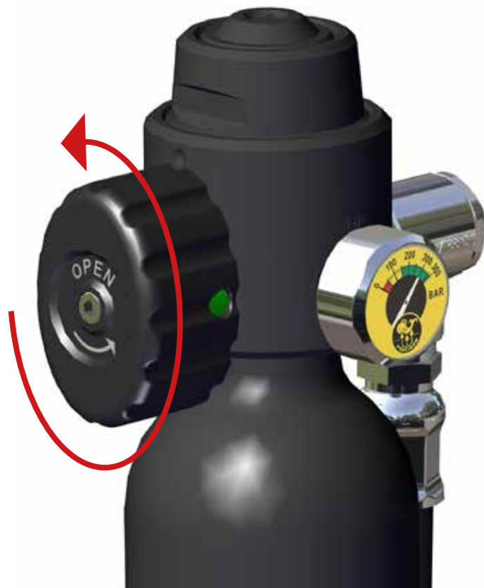
Cylinder valve in position OPEN Turning the valve handle counter clockwise until stop. Green color in the hole indicate OPEN position.
