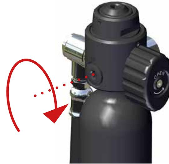
9. Mount the blanking plug in to the 7/16" HP port of the 1st stage and make sure it's firmly attached. Before mounting the blanking plug, inspect the o-ring to make sure it's without any flaws, make sure the o-ring is lubricated and that all sealing surfaces are clean and undamaged.
