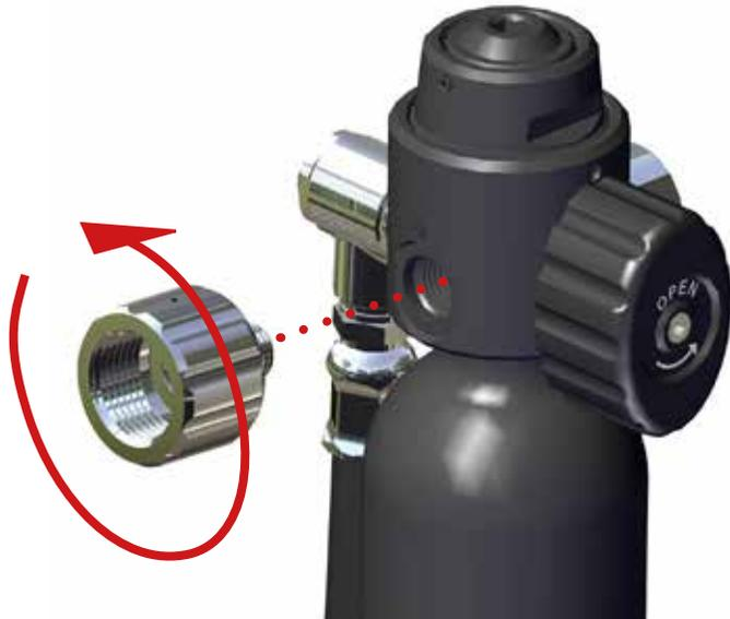
8. Unscrew the filling adapter/hose from the Poseidon EBS.
