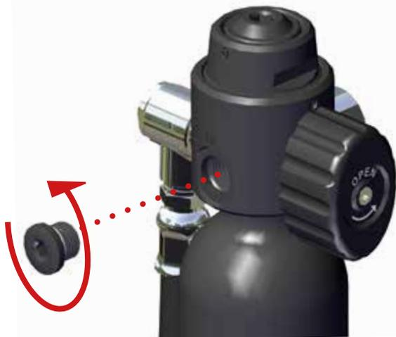
2. Remove the blanking plug from the 1st stage. Inspect the O-ring and attach the filling adapter to the 7/16" HP port where the blanking plug was mounted. Make sure the filling adapter is firmly attached. Attach the filling hose to the the filling adapter that corresponds to the max filling pressure stated on the cylinder neck.
