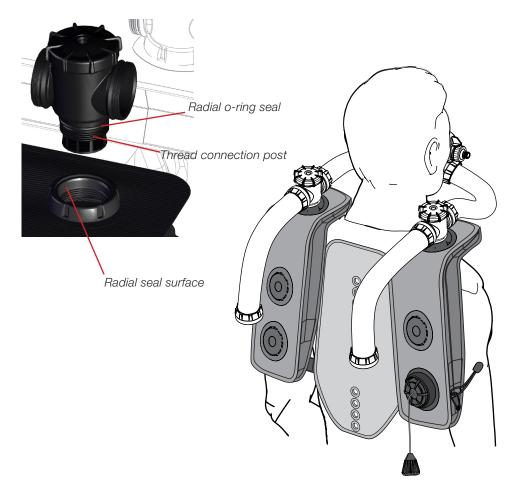
Insert the right hand water diversion manifold into the port on the right counterlung. Clockwise tighten the water diversion manifold into the right and left counterlung shoulder port.
