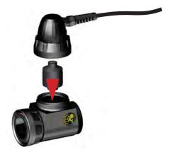
2. Connect the sensor lid to the POD (make sure the sensor is properly installed inside and the sensor's face is dry) and screw it in place. Connect the sensor cable to your off board external pO<sub>2</sub> monitoring computer and turn it on.
