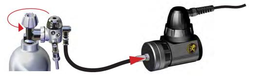
6. Connect the Manual Addition Valve (MAV) inflator hose to the nipple in the calibration lid earlier installed on the bottom of the POD and turn on the Oxygen tank valve on your MkVI or SE7EN. You will hear a hissing sound from Oxygen being injected thru the tiny flow restricting orifice inside the calibration lid.
